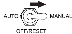
Figure 42. Auto-Off/Reset-Manual Switch (Manual Position)
